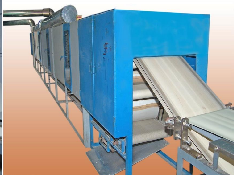
(2). Drier Machine ( Diesel, Oil , Gas ,Wood Fire Drier).
